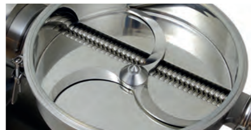
Flat-tray feeder with tray scraper
